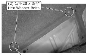
Install (2) 1/4" USS flat washers and secure using (4) 1/4-20 nuts with star washers
