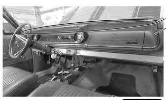
Remove (14) dash bezel mounting screws
