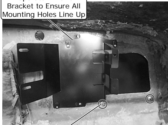
(2) 9/32" Washers and 1/4-20 Nuts with Star Washers
